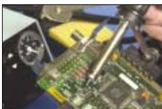
Non-contact soldering with the HAP1 hot air pencil.
