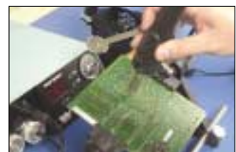
The DSV80 80-watt desoldering tool is perfect for desoldering through-hole components.
